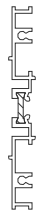
1G14 4 ½" Deep Adjustable Side Lite Base Vertical Mullion W/BRK. MTL. Use W/1G13 Horiz.
