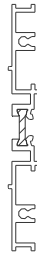
1G14 Adjustable Side Lite Base Vertical W/ BRK. MTL. Use W/ 1G13
