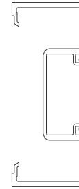
9212 Open Back Vertical 1/8" Wall for L102 Steel Use 9221, 9222 or 9246/FS93 Perimeter Adaptor
