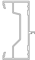
9232 Single Acting Door Jamb for Screw Spline Side Lites Use 9221 Glazing Adaptor Use W138 Weathering
